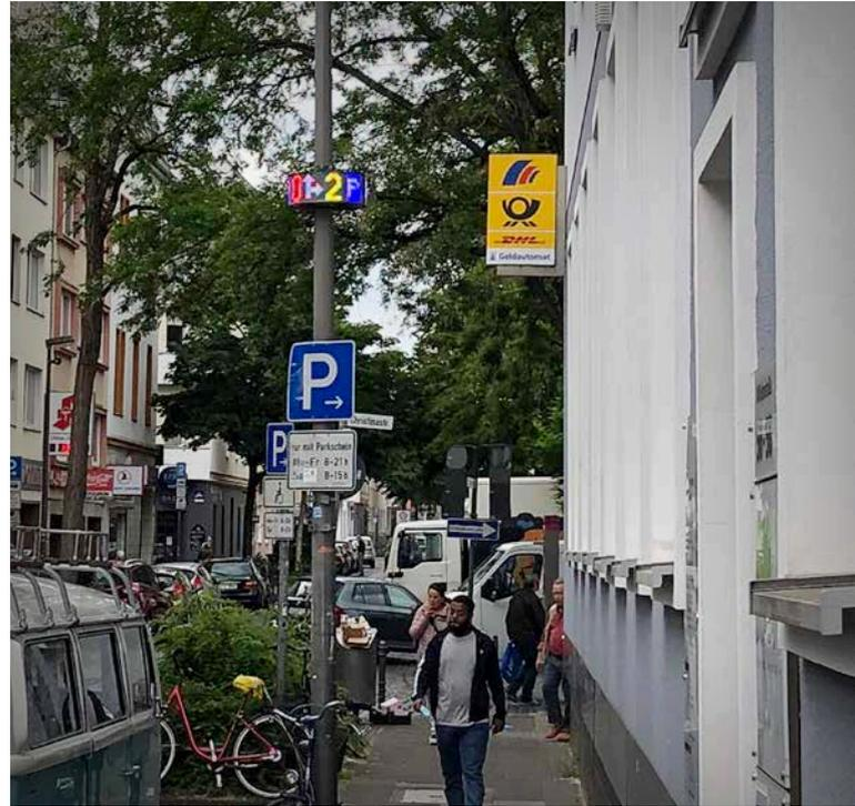
To avoid civil work on the surface and minimize disturbances in the neighborhood, the parking guidance system would have to be installed using the existing infrastructure of lampposts provided and managed by RheinEnergie.
