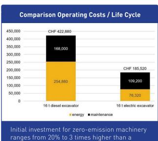
ranges from 20% to 3 times higher than a comparable diesel machine. However, electric machines have 40-70% lower operating costs. From a total cost of ownership (TCO) perspective, these savings nearly always compensate for the higher initial investment.
